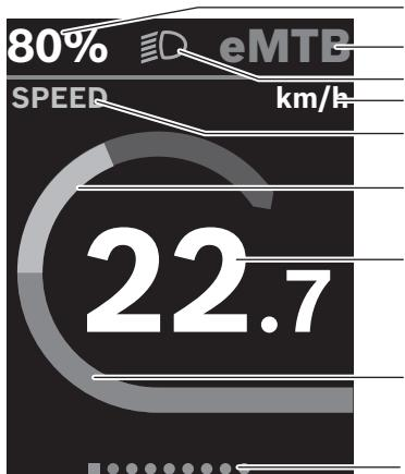
**a** eBike battery state of charge (can be configured)
